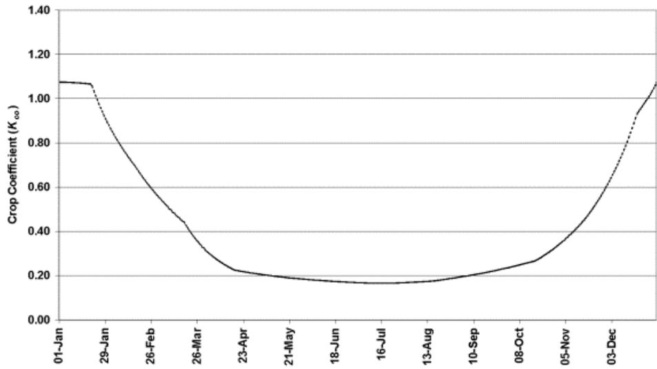
Figure 4. A plot of the annual  $K_c$  curve for bare soil for Fresno, California based on mean daily  $ET_o$  rate and days between significant precipitation ( $P_s$ ).
