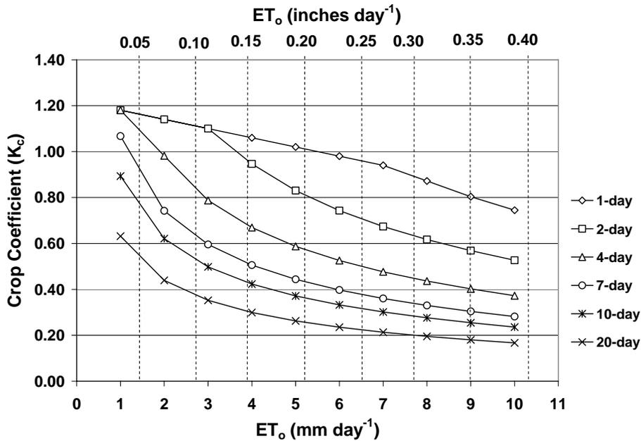
Figure 3. Crop coefficient ( $K_c$ ) values for bare or near bare soil as a function of mean  $ET_o$  rate and wetting frequency in days by significant rainfall or irrigation using a soil hydraulic factor  $\beta = 2.6$ .
