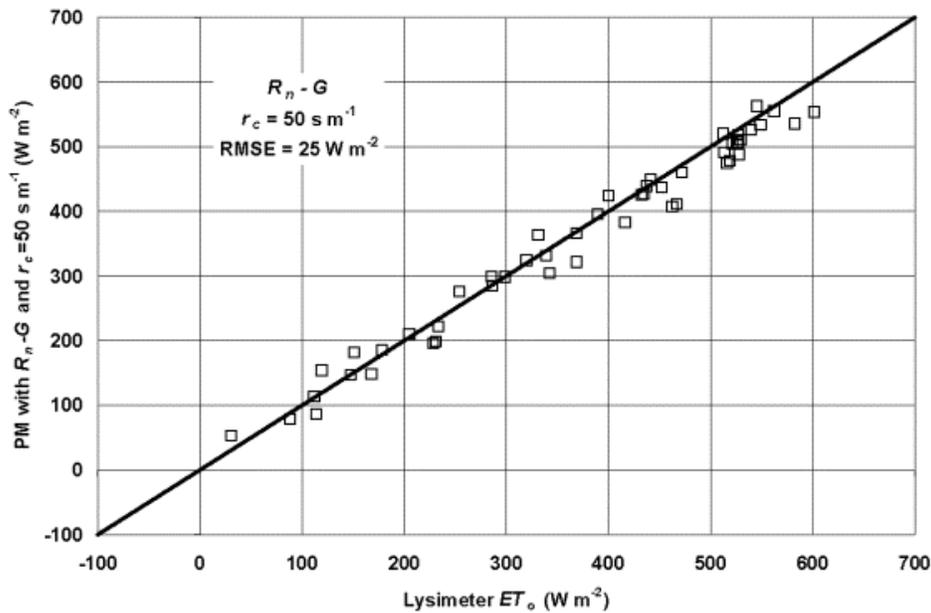
Figure 1. A plot of  $ET_o$  estimated using the Penman-Monteith equation with measured  $R_n$ ,  $G$ ,  $e_s - e_a$ , and  $u_2$  assuming a canopy resistance of  $50 s m^{-1}$  versus daytime, half hour lysimeter measurements of  $ET_o$ .
