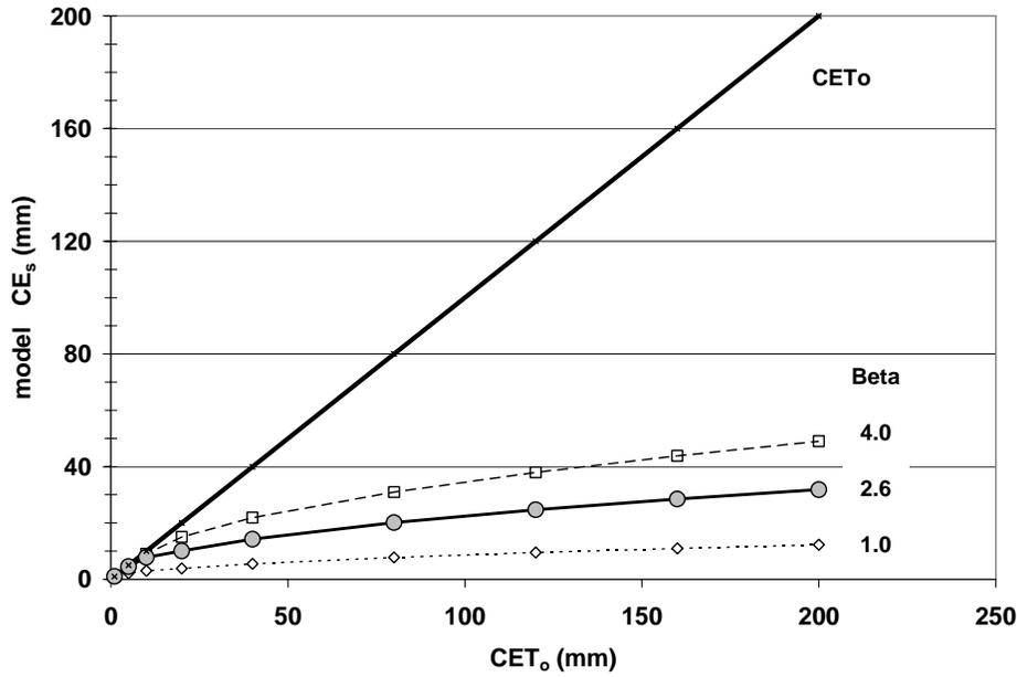
Figure 2. This plot shows the modeled cumulative soil evaporation ( $CE_s$ ) versus  $CET_o$  for three soil hydraulic ( $\beta$ ) factors.
