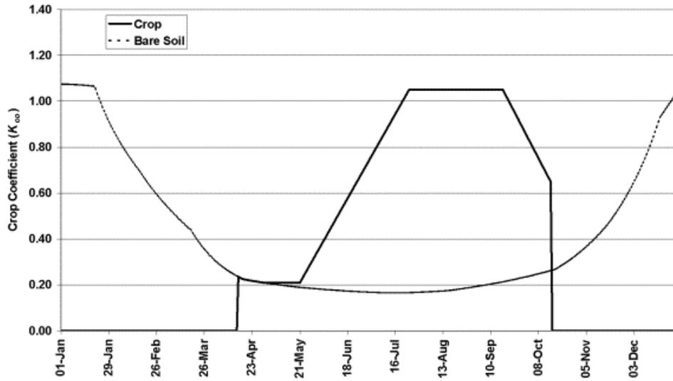
Figure 6.  $K_c$  curve, using a 30 day irrigation frequency during initial growth, for cotton grown near Fresno, California (solid line).  $K_c$  curve for bare soil (dotted line).
