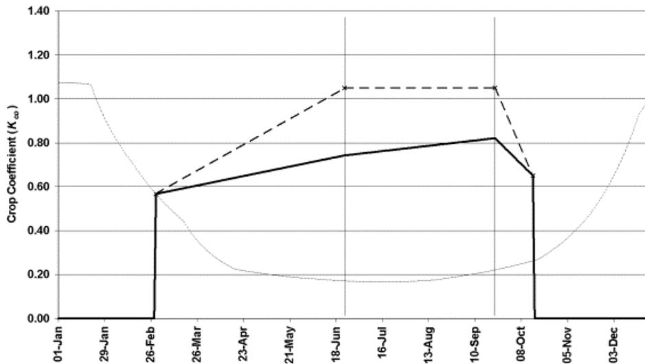
Figure 9.  $K_c$  curve for a stone fruit orchard grown near Fresno, California. The dashed line is for a clean cultivated, mature orchard and the solid line is for an immature orchard having  $C_g=35\%$  and  $C_g=40\%$  at the beginning and end of the midseason period. The dotted line is for bare soil evaporation.
