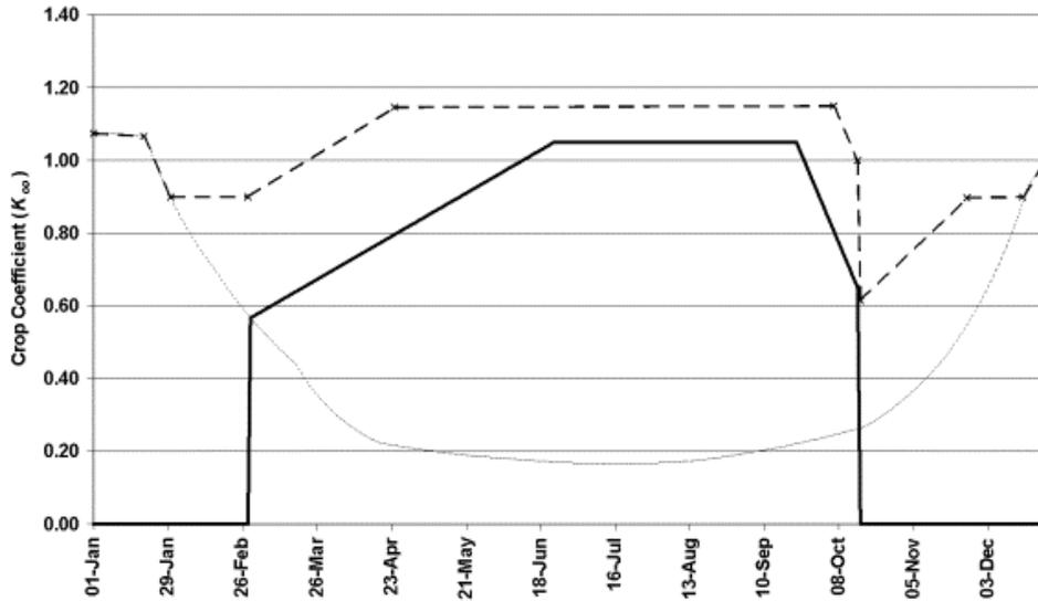
Figure 8.  $K_c$  curve for a stone fruit orchard grown near Fresno, California. The solid line is for a clean cultivated orchard and the dashed line is for an orchard with a green growing cover crop contributing a maximum of 0.35 above the clean cultivated  $K_c$ . The dotted line is for bare soil evaporation.
